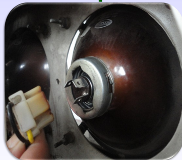
(6) Fit the bulb, lock the holder & connect the socket
