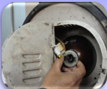
(2) Press & rotate anti clockwise to extract the holder
